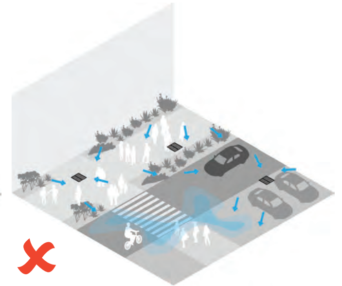
Fig. 59 - Drainage - What not to do Do not place gullies and drains in odd locations that result in twisted levels and pooling.
